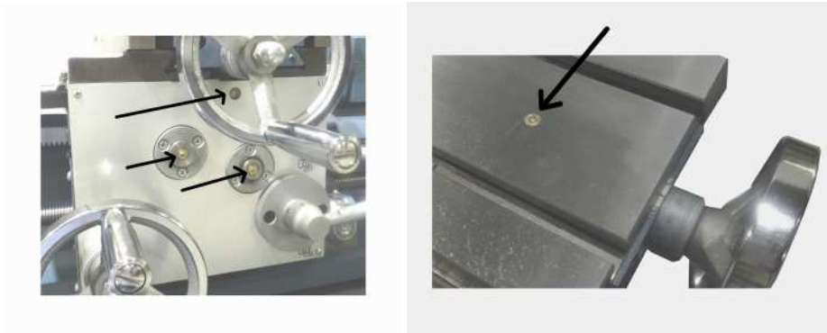
Figure 5.11 A & B Cross-Slide Screw Apron Oil Points and Cross-Slide Screw Table Oil Points
