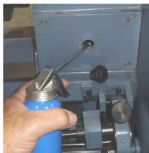
Figure 5.7 Add oil through the oil port located on the back side of the headstock.
