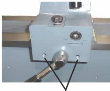
Figure 5.20 Gib Adjusting Screws - Tailstock (Shown with tailstock lock removed)
