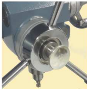
Figure 7.3 Mill/Drill Clutch pushed in engaging the Fine Feed
