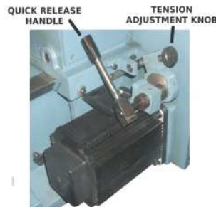
Figure 5.29 Adjusting Lathe Belt Tension - Shown in the down position
