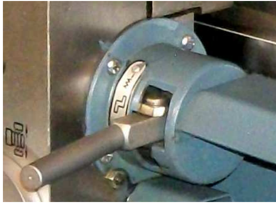
Figure 9.3 Powerfeed Engagement Lever Shown with Y-Axis powerfeed engaged
