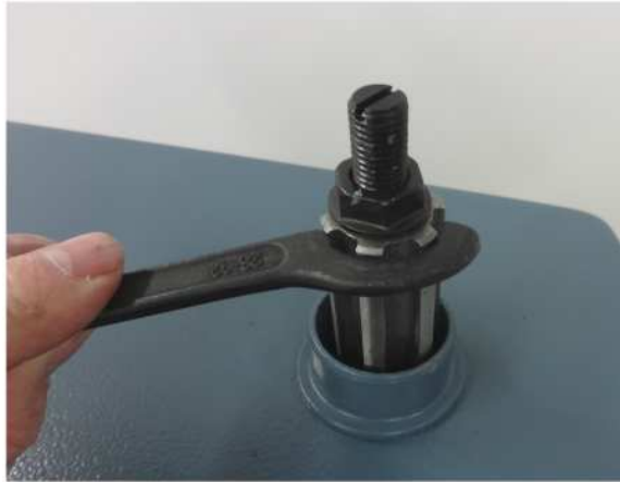
Figure 6.5 Use the supplied spanner wrench to hold the spindle in place while tightening the drawbar
