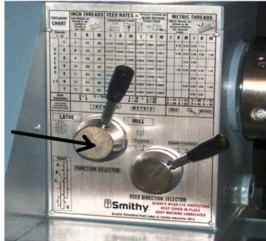
Figure 9.1 Always match the Powerfeed Function lever to the appropriate operation
