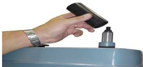
Figure 5.3 Installing Mill Spindle Cover
