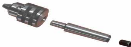
Figure 6.3 Install a plug into MT3 arbors when using them in the tailstock of a Granite machine
