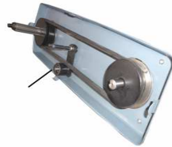
Figure 5.28 Adjusting Millhead Belt Tension
