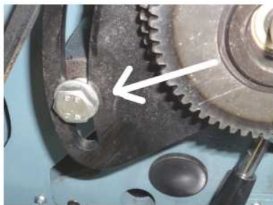
Figure 8.4 Loosen the bolt of the speed reduction pulley bracket when installing belts for the low speed
