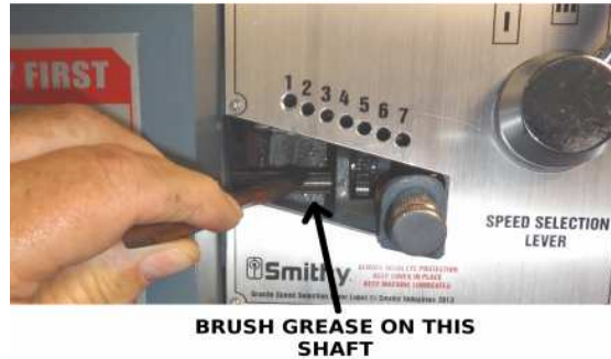
Figure 5.14 Oil the Quick Change Gear Box through the Powerfeed Slot
