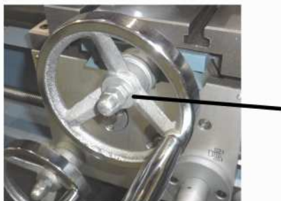
Figure 5.21 Loosen the two outer nuts holding the handwheel
