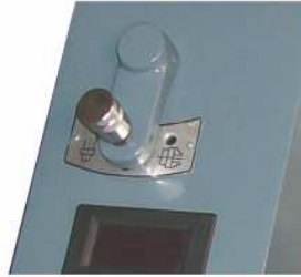
Figure 7.1 Lathe/Mill Clutch Shown in the Neutral Position
