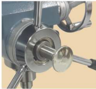
Figure 7.2 Mill/Drill Press Clutch pulled out, engaging the Drill Press
