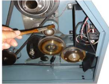
Figure 5.5 Brush a thin layer of lithium grease over the gear quadrant in the pulley box
