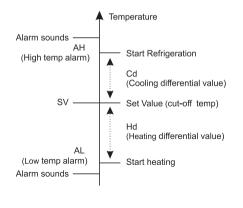
How it works: When the probe measured temp PV > SV + Cd, the controller turns on cooling equipment. The cooling indicator is on. If the indicator is flickering, it means the cooling equipment is under compressor delay protection status. When the probe measured temp PV drops and reaches SV, the controller turns off cooling equipment. The cool indicator is off. When the probe measured temp PV < SV - Hd, the controller turns on heating
