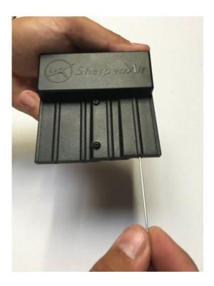
**Step 2:** This runner is at less of an angle than Step 1 and uses a less aggressive stone. Using the same amount of revolutions as step 1 (10-15), this step eases the angle even further in order to reach stock angle. This process will also help in removing some of the step one sand scratches.
