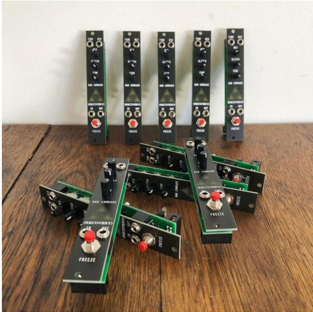
Freeze wrecked blips and oscillations in place, create scrambled gated delays, and straight-up over-the-top distortion, all mixed to taste with the original signal. CV available for mix and delay time.
