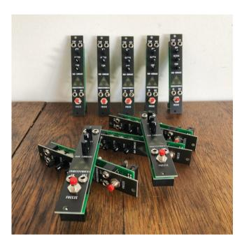
Freeze wrecked blips and oscillations in place, create scrambled gated delays, and straight-up over-the-top distortion, all mixed to taste with the original signal. CV available for mix and delay time.
