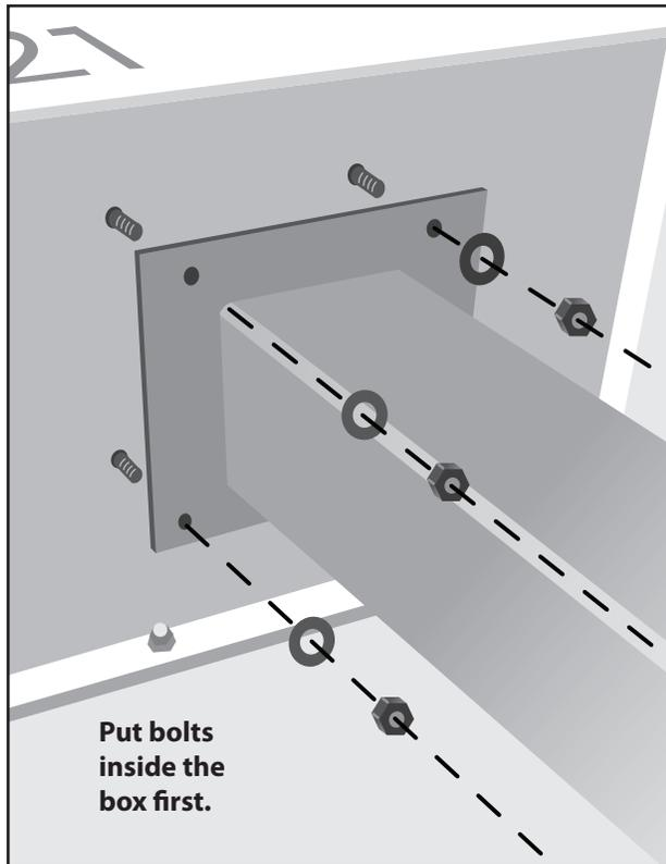
1. Attach the box to the pole with the four included 7/16" bolts, washers and nuts using your 7/16" Socket or Crescent Wrench.
