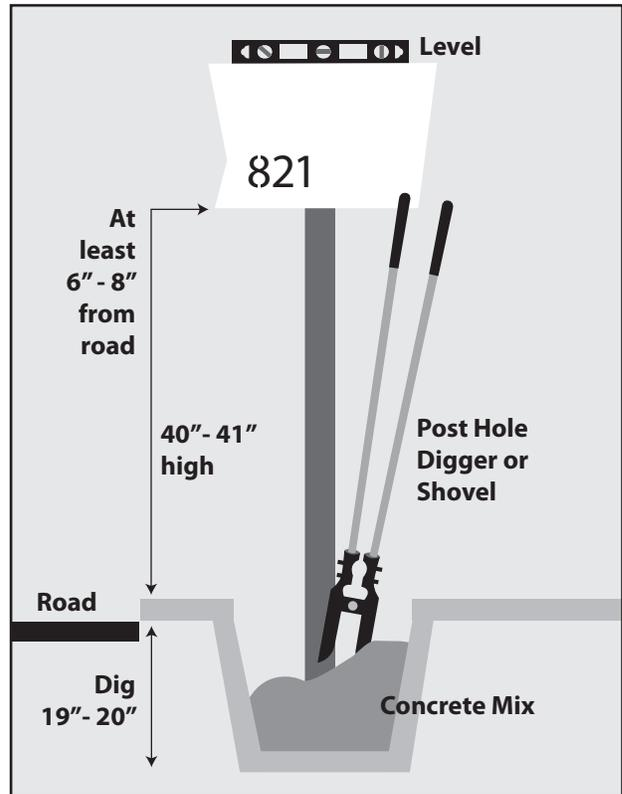
2. Place Pole with box attached in hole, and place level on top of the box. Level from front to back & side to side.
