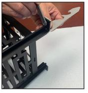
Use wrench provided to tighten locking screw.
