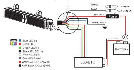
To connect without LED Control Module(LED-BTC), Connect as Shown in the Following Diagram;
