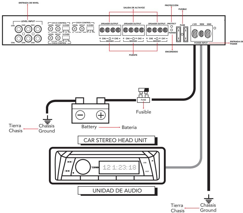
**IMPORTANT:** Before making any connections, disconnect the car's battery until the installation is completed to avoid possible damage to electrical system
