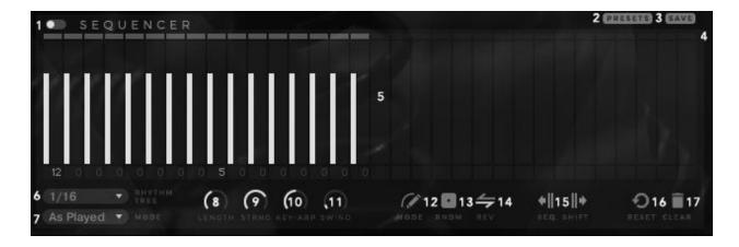
1. On - OFF. If the Sequencer is set to ON, it will begin stepping when the number of active voices goes from 0 to 1. Similarly, it will stop stepping when the active voice count goes from 1 to 0.
