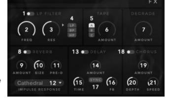
4. Filter Select (push buttons). Determines the filter whose parameter values are displayed, and gives an indication of which filters are active. Illuminated text = filter is on.
