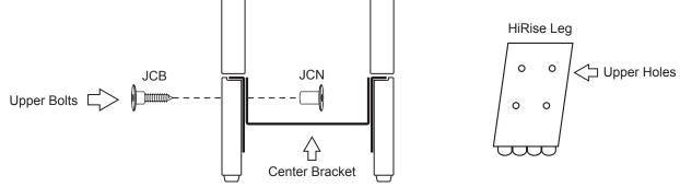
Using the remaining JCNs and JCBs, secure the Cross Brackets to the Down Bracket and wooden legs.
