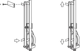
Ensure that the Down Brackets are orientated so the long flat side is on the inside of the rail as shown in the picture below.
