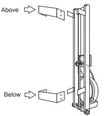
The long, flat part of the Center Bracket should be in a downward position. See pictures below for the correct orientation.
