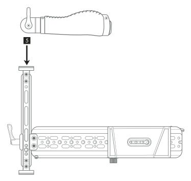
6. Loosen **THUMB SCREWS** to adjust **HANDLES** to desired position.
