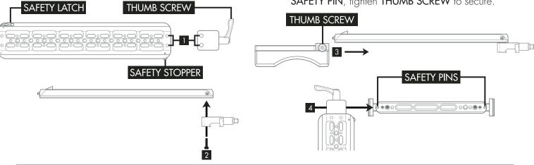
5. Select HANDLES, attach to CROSSBAR using THUMB SCREWS.
