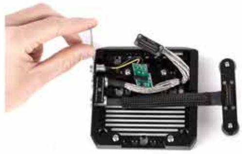
4. Using the included Fischer wrench, remove the Fischer nut from the Easy Top.
