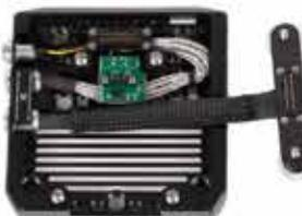
7. Using M2 socket cap screws, install the new module.
