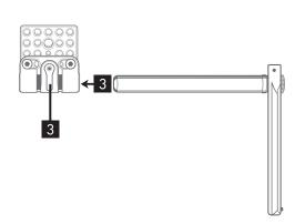
Select L-Bracket or EVF Adapter, install two #6 Screws and tighten to Knuckle using allen wrench. Slide Knuckle onto NATO Rail.
