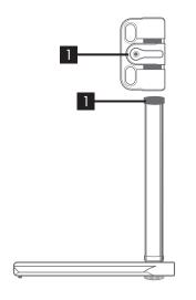
2. Locate two 1/4-20 Holes spaced between 25mm-36mm on Camera or Top Plate, select 1/4-20x3/8 Socket Caps, tighten screws to Tube Clamp using allen wrench.
