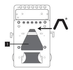
**NOTE:** Shim stickers can be added to Quick Back above Attachment Hole if necessary
