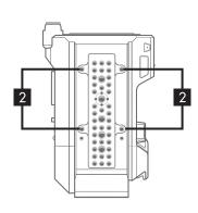
3. Select and tighten 1/4-20x1/2 Screws with allen wrench to secure Main & Center Plate assembly to Camera.
