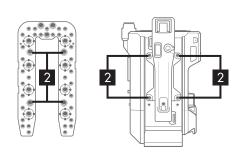
3. Select and tighten 1/4-20x1/2 Screws with allen wrench to secure Main Plate & Top Handle to Camera.
