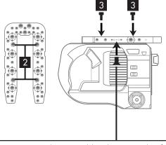
NOTE: To relocate Cable Clamp to side of Top Plate use M2.6x5 Screw.
