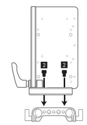
3. Attach Battery Mount using corresponding screws (see Hole Chart)
