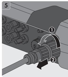
Disassembling the DC Connectors | DC-Steckverbinder demontieren | Демонтаж на DC
