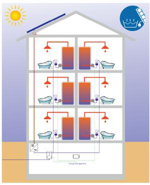
Decentralized hot water storage and production avoids distribution ("ring main") losses and fulfills hygienic standards.
