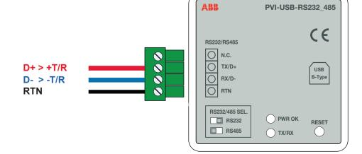
Insert the USB cable into the converter and in the PC
