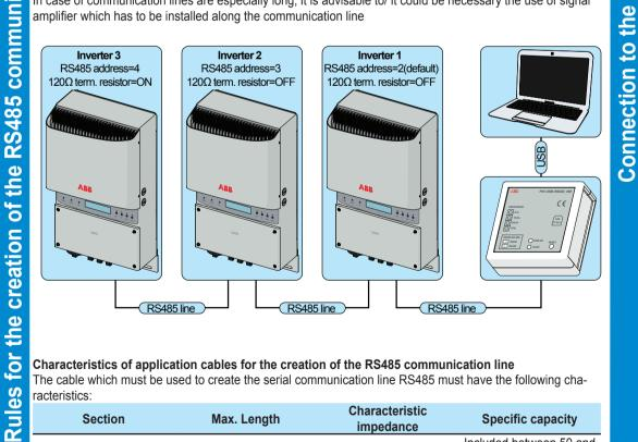
Characteristics of application cables for the creation of the RS485 communication line
