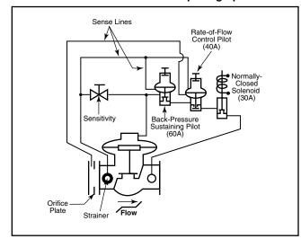
Model 200-60A-40A-30A Combination Back-Pressure Sustaining, Flow-Limiting, and Electrical Block
