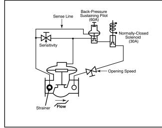
Model 200-185A-60A-30A Combination Back-Pressure Sustaining and Electrical Block with Opening Speed Control
