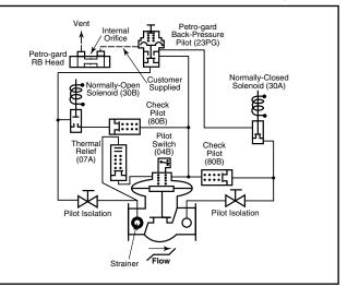
Model 210-80B/07A-23PG-04B Combination Digital Hydraulic Set-Stop and Back-Pressure Sustaining (Petro-gard) with Check, Thermal-Relief, and Position Switch
