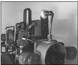
Model 04A Mechanical Position Indicator and Switch
