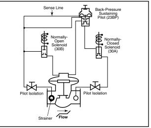
Model 210-23BP Digital Hydraulic Set-Stop with Back-Pressure Sustaining Control
