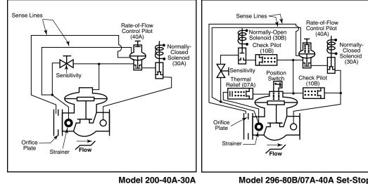
Model 200-40A-30A Combination Flow-Limiting and Electrical Block Model 296-80B/07A-40A Set-Stop with Flow-Limiting in Combination with Check and Thermal-Relief
