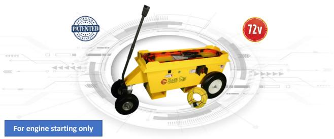
This American made jump starter is a larger version of the popular START PAC® 3324RR. This heavy duty 72V mobile unit is designed for engines up to 6000 horsepower or for multiple daily locomotive engine starting requirements. It will directly start the locomotive engine when the locomotive battery is not sufficiently charged or capable of starting the engine. The 3370RR will reduce operating costs by improving safety and efficiency in the field.
