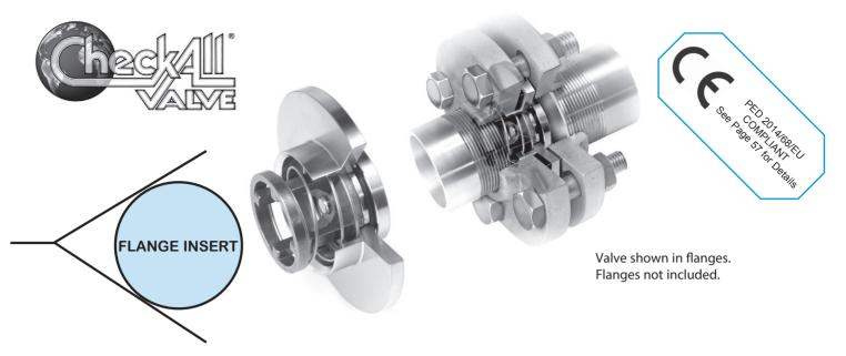
The **Flange Insert** (**F1**, **F6**, **FP**) valves are the ultimate check valve in flanged systems. They provide the simplest and most economical way to install check valves in a piping system. The valve body helps position itself while bolts are being installed and tightened. Two gaskets are required instead of the one normally used in a flanged joint. See page 53 or consult the factory for additional installation guidelines.
