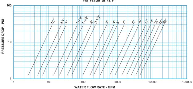
Flange Insert Flow Curves assume Schedule 40 pipe For Water at 72°F
