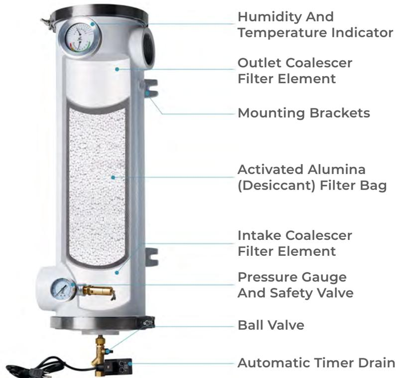
Super-Dry Compressed Air Dryers contains two highly efficient polypropylene coalescer elements at inlet & outlet ports to absorb oil and all solid air particles. Also included, one desiccant bag specifically designed to absorb water vapors and humidity from your compressed air system.
