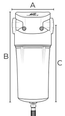
Maximum inlet temperature: 176°F (80°F) Maximum inlet pressure: 232 psig
