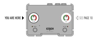
Punishing voltage and input sensibility (see page 10) can be defined at the same time by entering the same procedure described in steps 1 to 5 by pressing and holding the ON/OFF footswitch.
