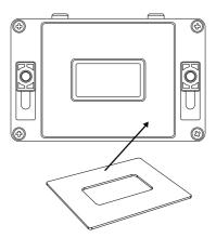
2 Loosen the 2 thumb screws to unlock the bottom pieces out of the pedal.
