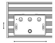
Tighten the two thumb screws with your hands or with a screwdriver.
