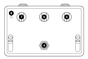
**6 TONE**: The original Vox UL series amp's fuzz had a preset low pass filter. We've replaced the fixed resistor in that part of the circuit with a potentiometer so you can make it sound brighter or darker depending on the instrument and/or amp you're playing. Turn it clockwise to make it sound brighter.
