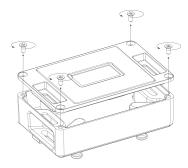
3 Put the 9V battery in the position showed in the diagram. Make sure to use a good quality alkaline battery to ensure the longest time of operation.
