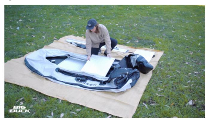
The bow section goes in first, then the second piece and so on. Be careful not to pinch any part of the hull material.
