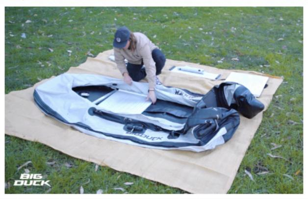
The next step is to lay the floor panels inside the hull. These lock into each other with a tongue-in-grove style system.
