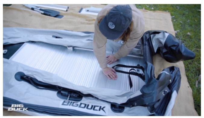
Carefully push down on the risen join until flat. This will lock the panels into place and also tension the length of the hull. Be sure to have all panels in the correct location before pressing down.
