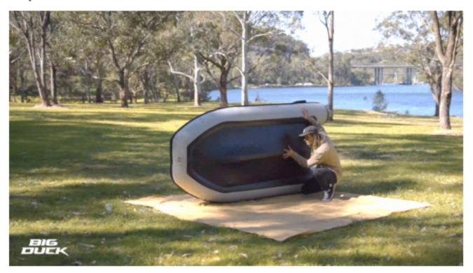
Check that all valve caps are secure and then lift the hull up onto on side to ensure that the keel is centred. Your keel will help provide stability.
