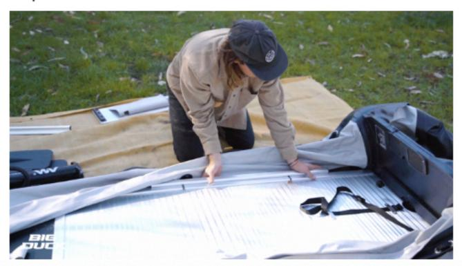
Next, secure the first side joiner. These overlap the rectangular panels and help give the floor its rigidity.
