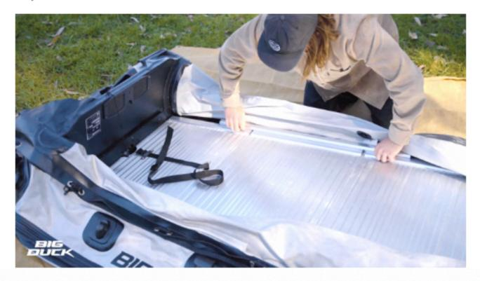
Then secure the opposing side joiner, repeating the same process and ensuring that both joiners are evenly positioned.
