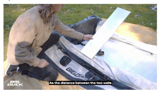
Attach the bench seat. This attaches using a track system that slides into place and is then adjustable. Attach both sides before the next step.
