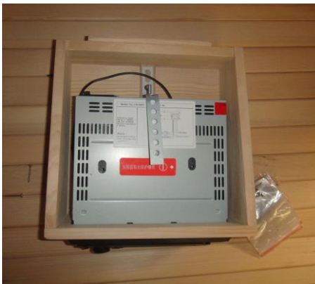
FIG-15.1 Radio Player in wood housing
