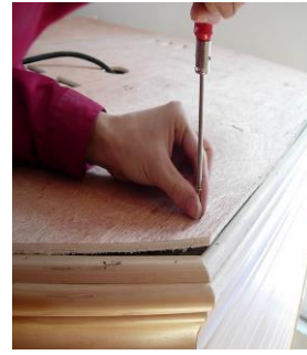
FIG-18.1 Screw down Roof Cover
