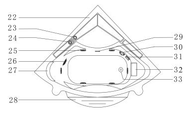
22. Bathtub28. Marble23. Air adjuster29. Bottom light24. Air switch30. Steam outlet25. Water jet31. Drainage switch26. Water inlet32. Waterfall27. Pillow33. Drainage
