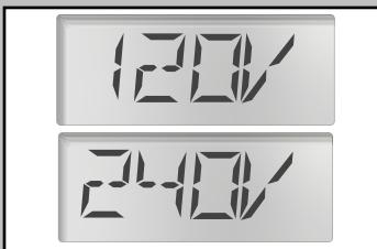
Make sure the voltage shown on your screen matches the electrical voltage of the hot tub (**120V OR 240V**)
