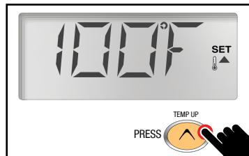
Pressing the "TEMP UP" button or the "TEMP DOWN" button will cause the current set temperature to flash
