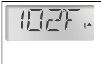
When the flashing stops, the temperature is set and will show the current temperature of the water
