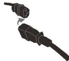
FIG-14 Connecting cord connectors
