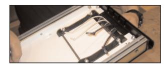
2. Take both light and heavy cords and slip both through the rollers at the opening at each end. Make sure the cords are at the right position according to the arrows on the label. Notice 2nd roller set is different from older SRF boards
