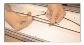
3. Pull each cord to overlap 2 inches. Use the Zip strap to tightly secure the tension cords together. Repeat steps 2 -4 for the remaining 3 tension cords. Use scissors to cut the loose ends of the zip straps off. As cords stretch out over time, extend the over lap which effectively shortens the overall length of the cord.
