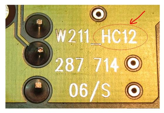
It means you have **912** CPU. Do make a jump like in picture (you can keep this jump even after reading/writing finishing).
