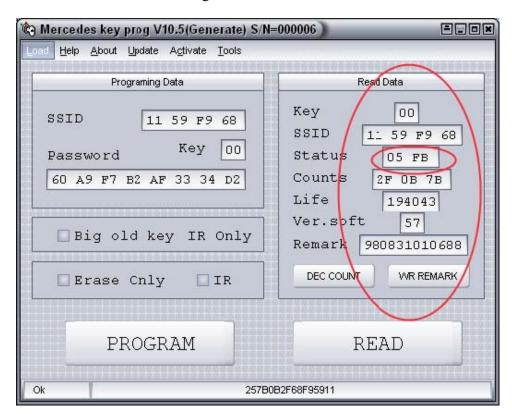
Status **05 FB**, this key is not activated yet. If you need to activate it before inserting in to EZS (only for old type EZS based on HC05 CPU) press Activate bookmark and choose type of work: IR (via Infra Red port, if you already put CPU back on the key board) or PCB (if CPU still on adapter board).
