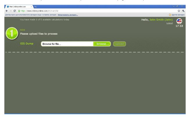
You have to upload Motorola EEPROM data from EZS: external CPU HC05 from old type EZS, CPU HC08 with key data, CPU 912 or 9s12. No need to select exactly CPU type. The software detects it itself.
