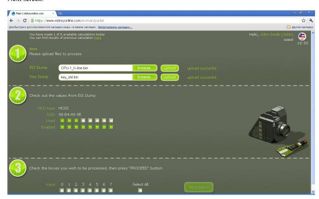
For this old type Motorola CPU you can see only name of type (HC05) and SSID after uploading. There are three active (Used) keys – numbers from 00 to 02. "USED KEY" means that with this key they started this car at least one time. You can see that all 8 keys are available for calculation (Enabled). If this EZS has locked keys (disabled) their positions painted by red.
