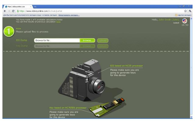
If you going to work with old type EZS (like in picture) based on two Motorola CPU HC05 series and you have at least one key (old type, Motorola HC705E6 based) from exactly this car you can read CPU1 eeprom by K-line (diagnostic connector) without taking it off. It's better to do it with our MB KEYPROG 2 or MB KEY RESTORER.
