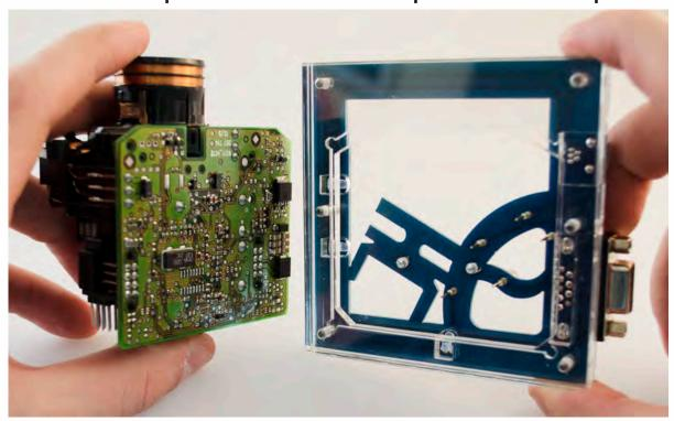
Carefully put the bottom of EIS into Click'n Go adapter.
