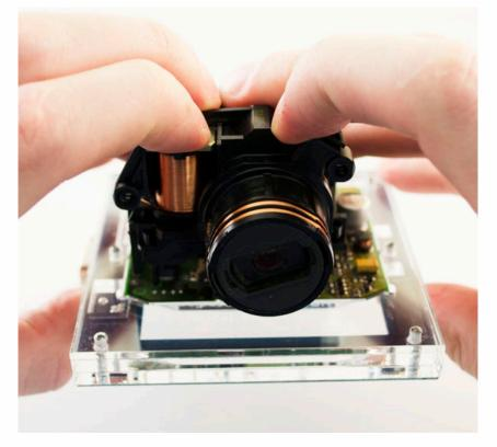
Make sure that Click'n Go adapter is mounted correctly on the EIS.
