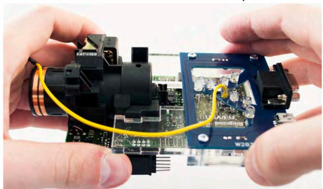
Carefully Push the corners of EIS board on to Click'n Go adapter.
