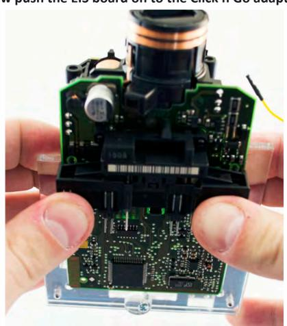
Secure EIS with the safety locks by rotating it over the board.
