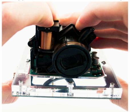
Make sure that Click'n Go adapter is mounted correctly on the EIS.
