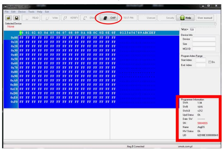
Make sure that JTAG is selected in programmer software. Select MOTOROLA > MC > HC12/HCS12/HCS12X > SECURED > EEPROM and double click on MC9S12 EE SEC option as seen in the red circle.
