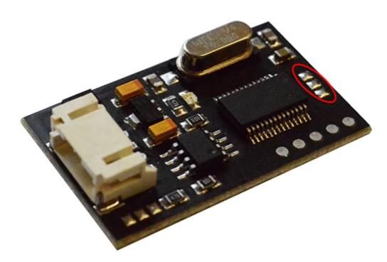
Set contains additional resistor that can be soldered on the marked place (pin 1 and pin 3).
