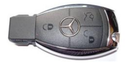
In case you deal with a "green key" in this version (can be found more seldom) you may work via IR without disassembling the key (which is preferable as it is simpler) but as it is possible to work through PCB board (having soldered off the processor) we have kept this function in our program.
