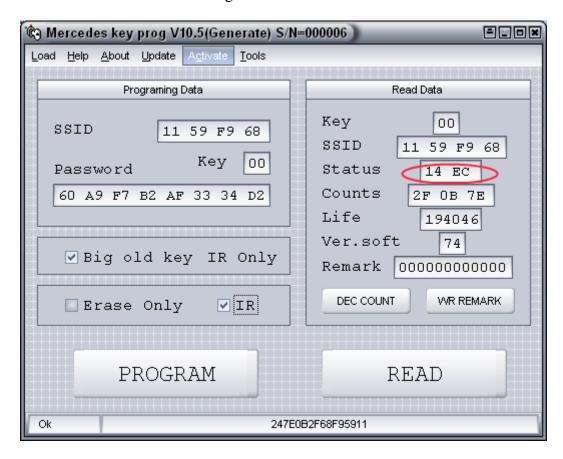
When programming the keys based on MOTOROLA processors via IR-ports you must remember what kind of processor is in the key. The programmer will solve this problem. You simply choose the preprogrammed EEPROM dump format of the file you load.
