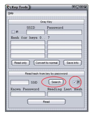
The device will read SSID of the key and if SSID is in your base you will see the password in the right field
