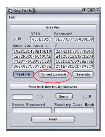
By pressing this button the "green key" will be converted and can be used further as a normal key.
