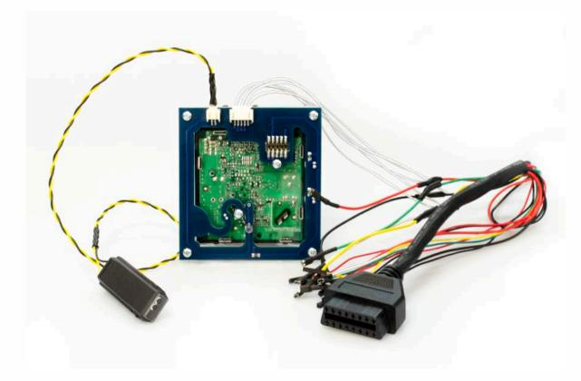
Connect Magic Eraser to the cable and power it up with 12V battery.
