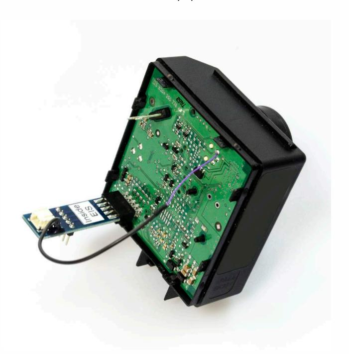
Connect Magic Eraser SE cables to the adapter PINs. Make sure that the cables are connected in a right way (Instructions are on the outside of adapter).
