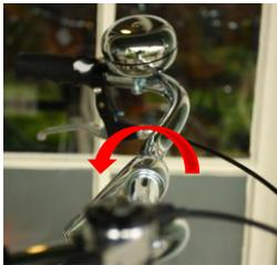
To adjust handlebar tilt, use a 6mm hex key to loosen the bolt on the front of the stem attachment, then rotate the handlebar until the desired angle is achieved. Ensure the handlebar is centred before retightening.
