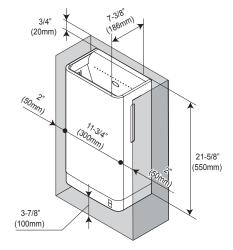
\*\*\*Clearance is required in order to take the water tray side covers for cleaning and maintenance.
