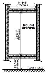
Recommended framing: Prepare wall opening using double stud and according to the picture measurements Min opening depth: 4-5/16" (110mm)
