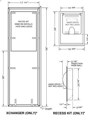
Both the XChanger (STD Height) and Recess Kit 3366139 are included with Combo Kit 3366135
