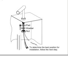
4.Position the mounting template at such a place that the soap tube can reach the gray circle on the mounting template.
