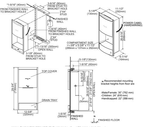
\*WALL THICKNESS REQUIREMENT: MIN 3/16 in (5mm) TO MAX. 1-3/16 (30mm)
