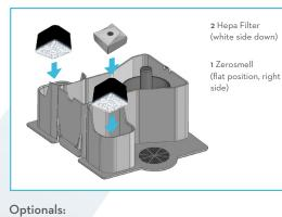
The basic maintenance consists in emptying the water tank and cleaning the air filters following the instructions of the user's manual. An electronic device warns (audible and visual alarm) if maintenance is required.
