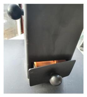
8. The stove may leak smoke from the side vent or top lid at the start of each burn. Ensure that you are in a well-ventilated area. If the damper gauge in the flue pipe is not opened fully, the stove will noticeably leak a lot of smoke. Learning how to manage the damper is vital to the operation of the stove! Check the flue pipe exit regularly whilst burning to ensure that the fumes are flowing freely from the built in spark arrestor.
