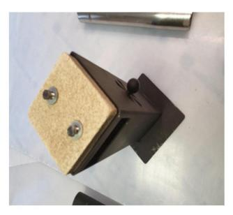
4.Install the bottom plate with the previously removed screws. Ensure that the counter sunk holes are facing you.
