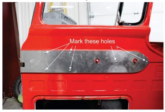
Mark the holes on the inside panel of the door. These will be drilled using a 3/16" drill bit.
