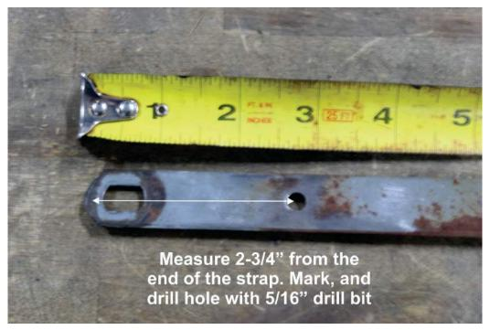
Measure 2-3/4" from the end of the steel strap and drill a 5/16" hole.
