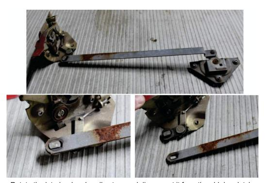
Rotate the interior door handle strap and disconnect it from the old door latch.
