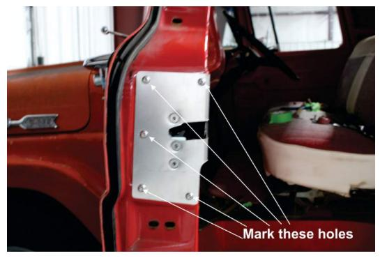
Mark the holes on the outside edge of the door. These will be drilled using a 5/16" drill bit.
