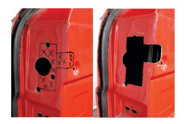
Carefully cut away the marked off area using a reciprocating saw or cut-off wheel.
