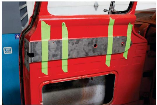
Locate your installation panel and place it on the door. Center the panel to the raised interior part of the door and make sure the latch area is seated firmly against the door. Secure panel with tape.
