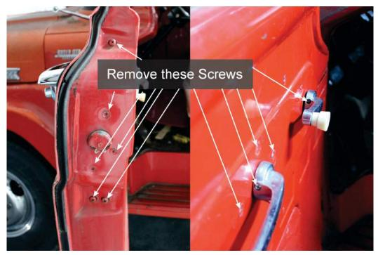
Remove the 3 screws holding your window channel, along with the 4 screws that hold in your door latch. Remove the interior door handle and window crank by loosening the set screws that hold them and pull them off of the regulator shafts. Remove the 3 screws that hold the interior door handle regulator to the door. Remove the door latch, interior door handle regulator, and the steel strap that connects them, all as one piece through the access hole in the door.
