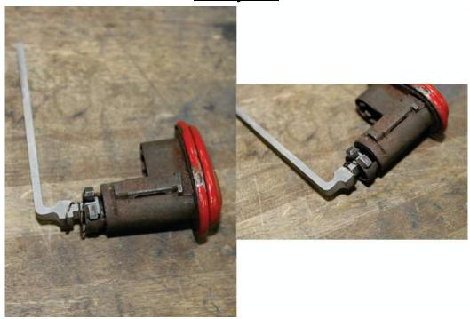
On the back of your truck's lock cylinder, depress the spring and remove the lock lever. Replace the factory lock lever with the new lock lever supplied in your kit.
