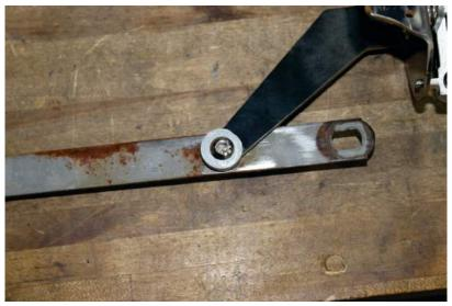
On the inside of the door, attach the steel strap to the latch lever using the ½-20 bolt, (2) ½" flat washers (one on each side of the strap), and ½ locking nut.
